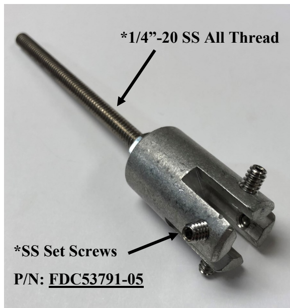
Figure 24: 4-Point Anchor with SS Set Screws and 1/4"-20 SS All Thread Studs (4-Point Anchor Assembly)
